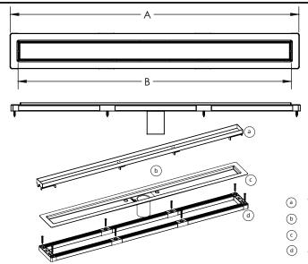
GRATE CAN BE ADJUSTED UPWARDS AN ADDITIONAL 1/2"
