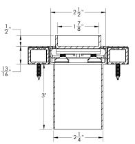
GRATE CAN BE ADJUSTED UPWARDS AN ADDITIONAL 1/2"
