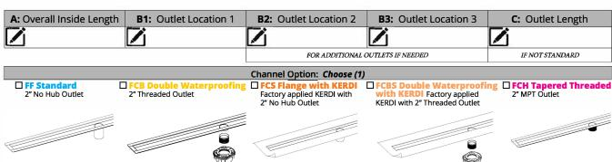
Note: Lengths exceeding the grate's maximum single length will be split into equal sections.
