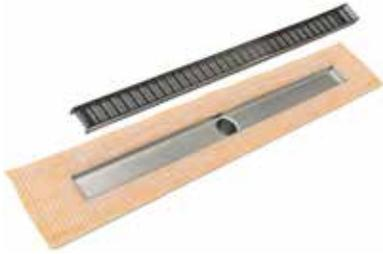
FCS Series linear drain kits are compatible with all grate styles and feature a pitched channel in a set length with a center outlet and factory applied Schluter®-KERDI fabric. These linear drains are compliant with the Schluter®-KERDI shower system warranty and backed by the Infinity Drain warranty.
