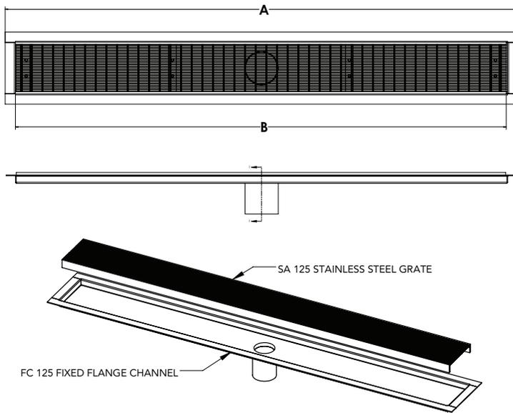
GRATE CAN BE ADJUSTED UPWARDS AN ADDITIONAL 1/2"
