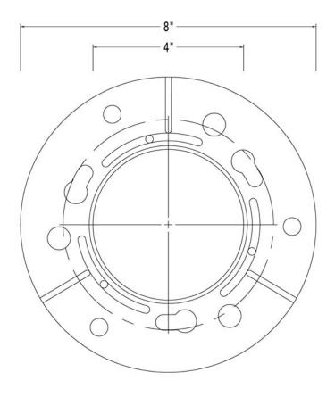
Universal 4" Clamping Plate, 8" overall diameter x 4" throat.
