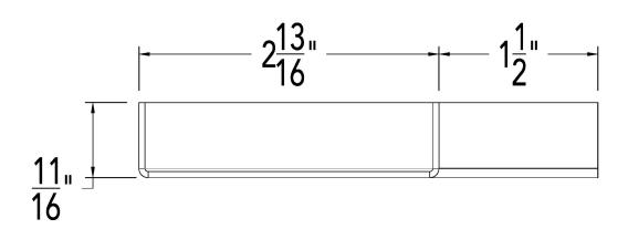
Stainless steel angle joiner for 90° installation for SC/LC Channel
