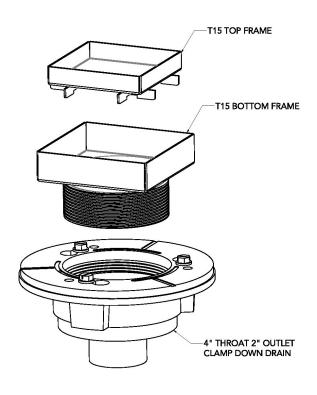
TD 15-2I 5" x 5" Kit with Cast Iron Drain Body No Hub Outlet
