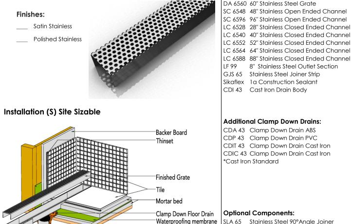
Waterproofing membrane Sub-floor Threaded Outlet Assembly Joiner Strip Channel
