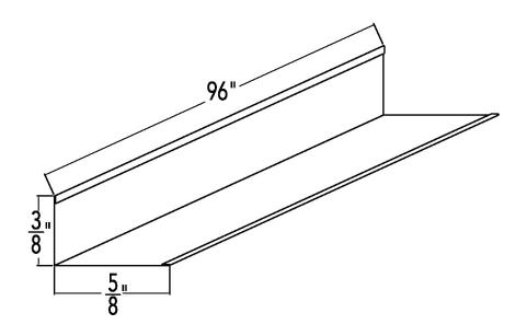
Tile Edge Profile for FF + FT installations.  $3/8 \times 5/8 \times 96$ "
