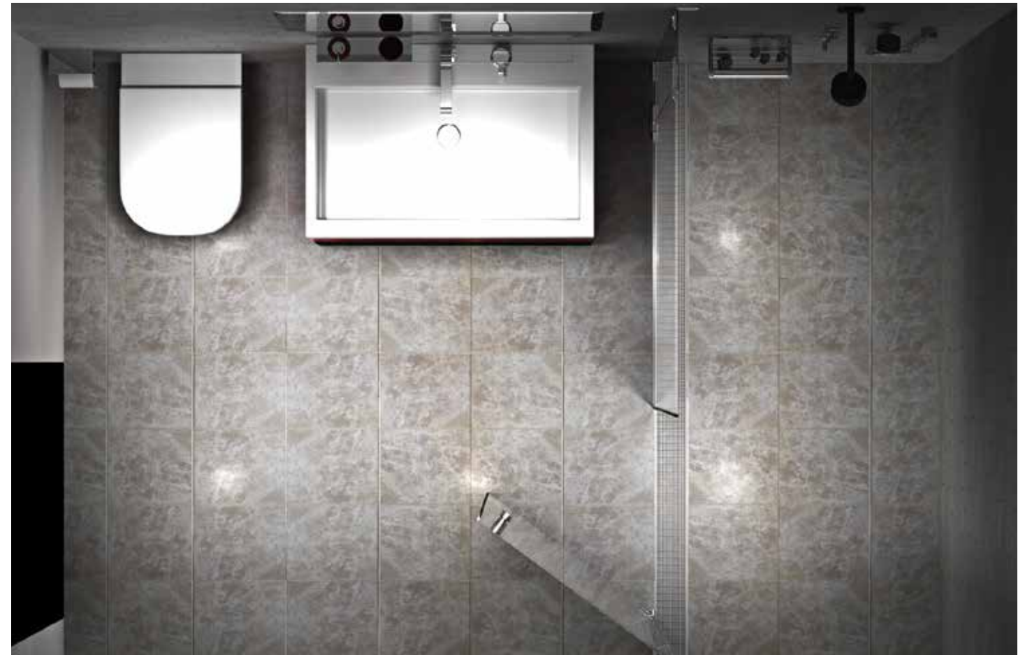
Barrier free zero-threshold installation. The entire floor is sloped toward the linear drain. Both 'wet' and 'dry' areas are waterproofed.
