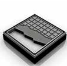
Size 5"x5" 16 gauge, 304 Stainless Steel ABS/SS Body 2" Throat Installation Types: Center Drain (TD) Center Drain (TDB)
