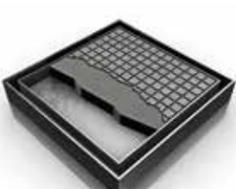
Size 8"x8" 12 gauge, 316 Stainless Steel Stainless Steel Body 4" Throat Installation Types: Center Drain (TD) Center Drain (TDB)
