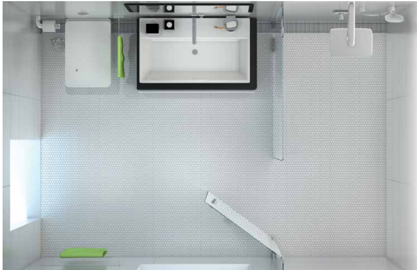
Create a wet room by running the linear drain along both the 'dry' side and 'wet' side of the bathroom. The entire floor is waterproofed and sloped toward the linear drain.
