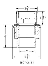
2 INCH CLAMP DOWN ASSEMBLY NOT INCLUDED IN KIT SKU (MATERIAL CAN BE CAST IRON, ABS, OR PVC)
