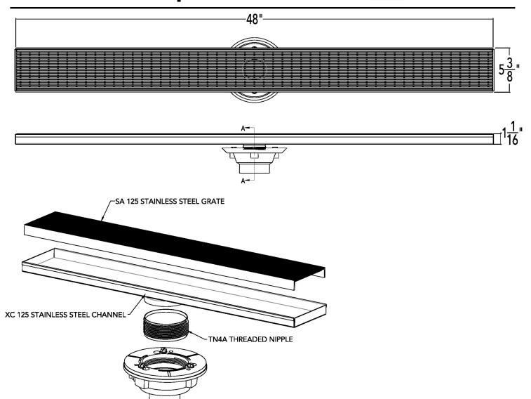
3 INCH CLAMP DOWN DRAIN ASSEMBLY (MATERIAL CAN BE CAST IRON, ABS OR PVC)
