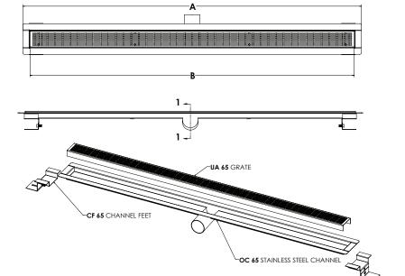
Grate can be adjusted upwards and additional 1/2"
