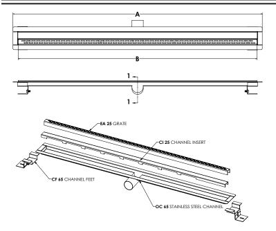
Grate can be adjusted upwards and additional 1/2"
