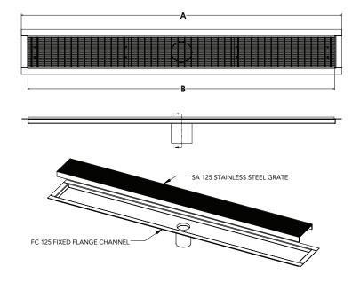
GRATE CAN BE ADJUSTED UPWARDS AN ADDITIONAL 1/2"
